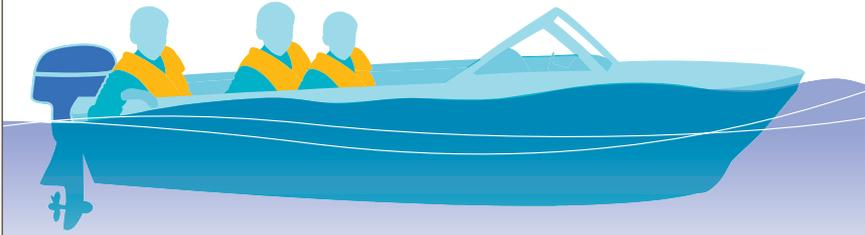
Level flotation means the boat will continue to float in an upright position if swamped. This will allow you to remain in the boat and bail the vessel to remove the water.
