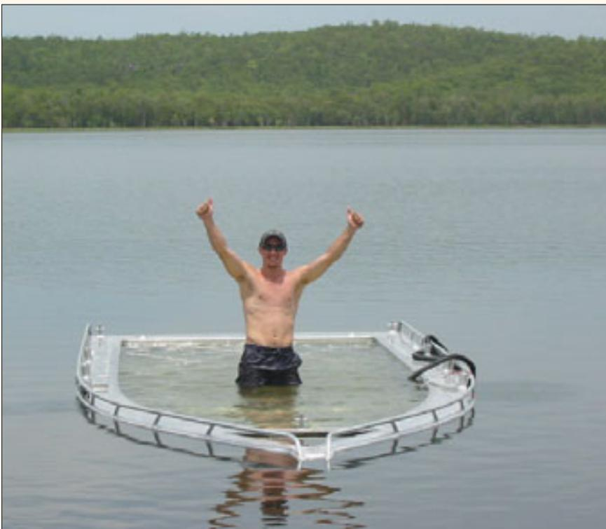
**Left:** Here is an interesting photo of the Hydracraft 660 Pro Guide by GS Marine in Darwin NT undergoing swamp tests to determine the level of the flotation (and stability) of the boat when it has been swamped, and filled with water.
