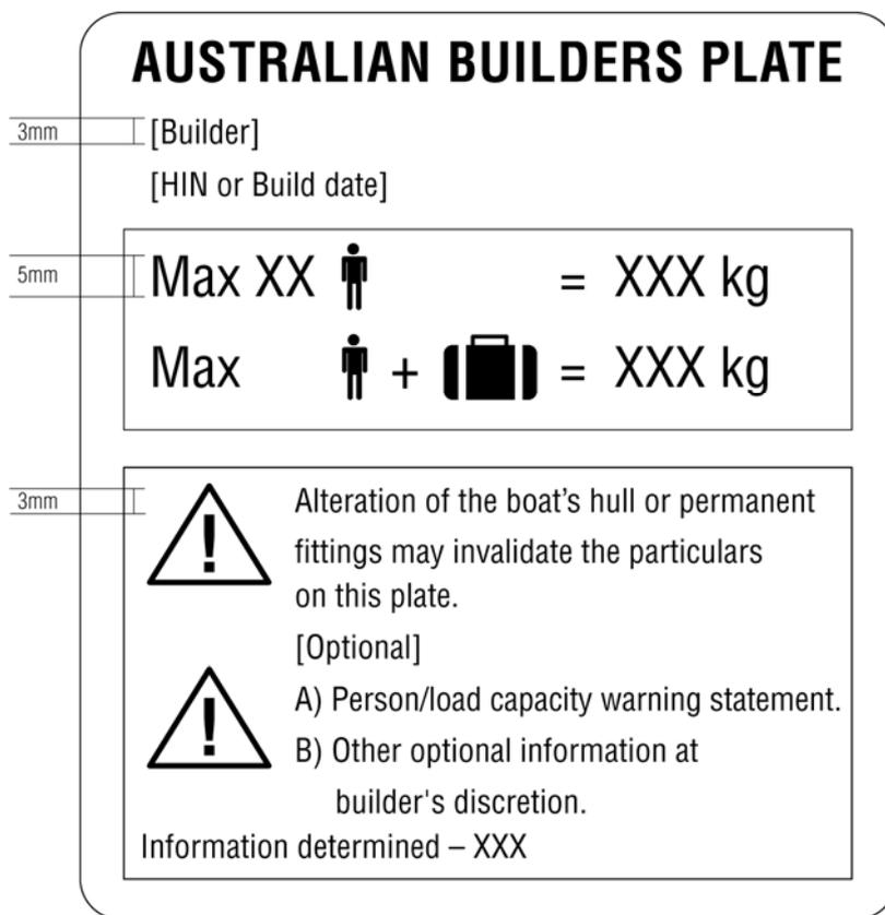
**Figure A.8—Sample ABP template for boats 6 metres or more in length, not designed to be powered by an outboard engine using text and symbols**
