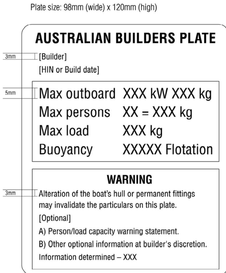
**Figure A.1—Sample ABP template for boats less than 6 metres in length designed to be powered by an outboard engine**
