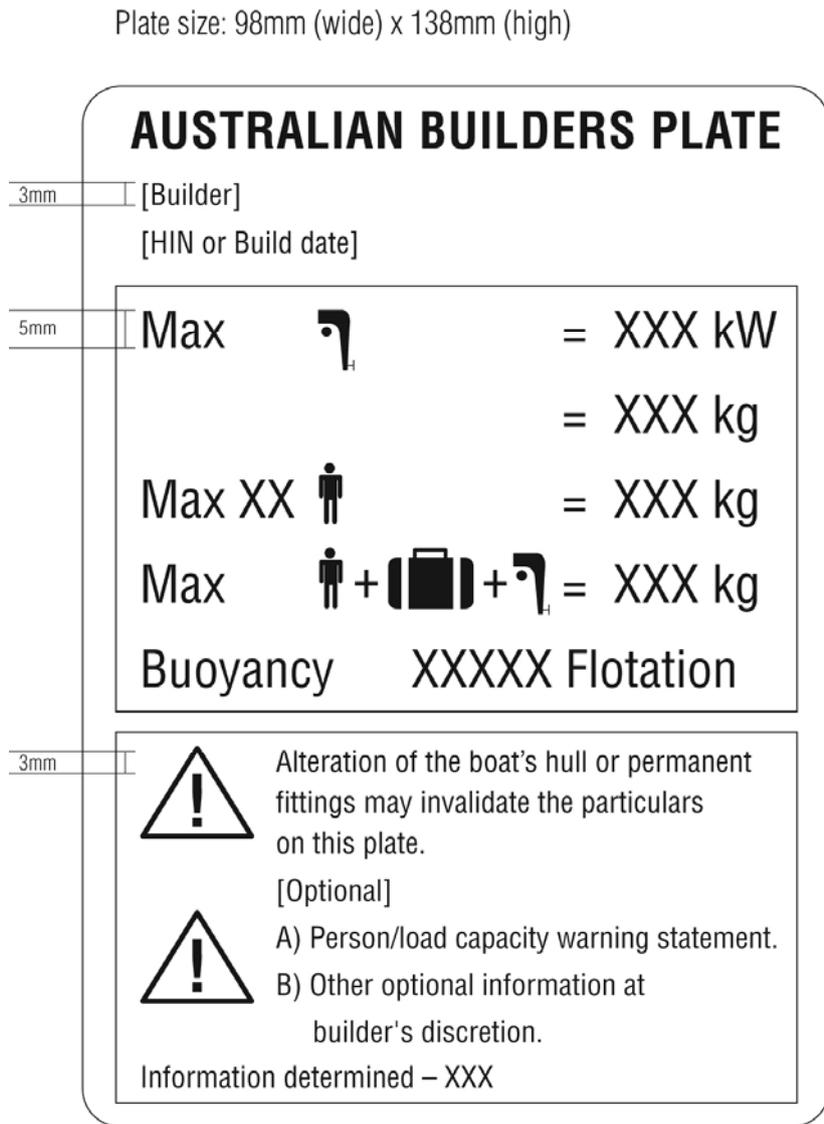
**Figure A.3— Sample ABP template for boats less than 6 metres in length, designed to be powered by an outboard engine, using text and symbols**
