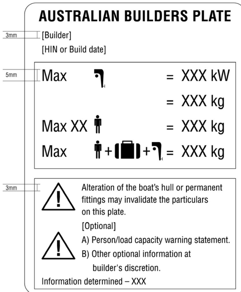
**Figure A.7—Sample ABP template for boats 6 metres or more in length, designed to be powered by an outboard engine, using text and symbols**
